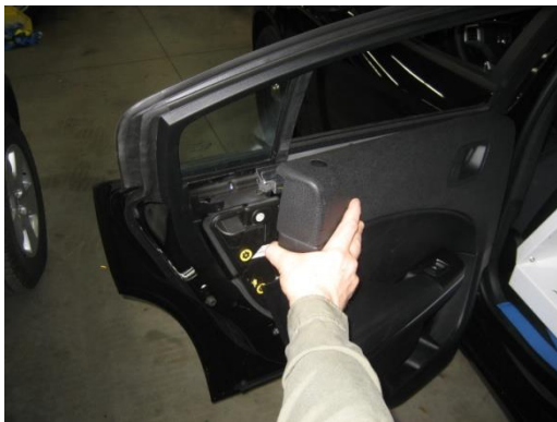
Remove / unsnap entire door panel from door. (Use Trim removal tool to pop clips)
