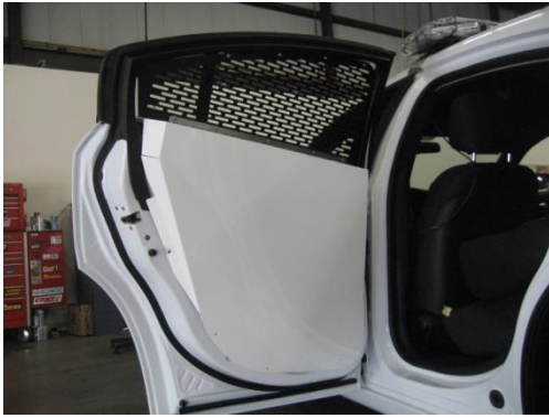
Door panel and Window guard complete. Proceed to the other side. NOTE: It is very important to double check door lock operation prior to closing door.
