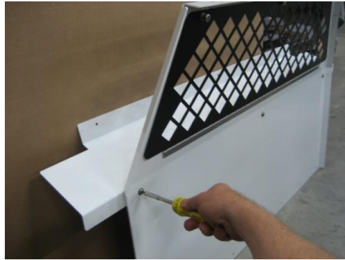
Attach rear upper support / mount bracket to the rear wall with 1/4" x 3/4" Phillips pan head screws and flat washers.
