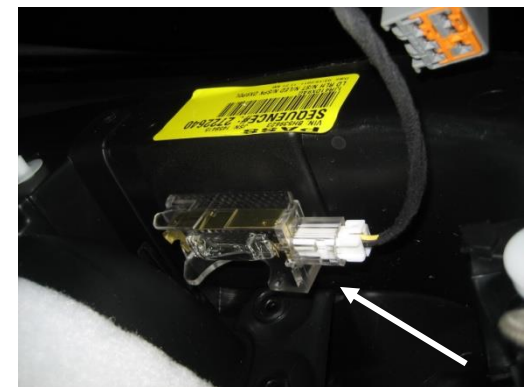
Unplug ground light wire from bottom of door panel.
