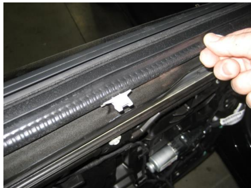
Attach rubber / felt glass wiper edge molding back onto metal door flange.
