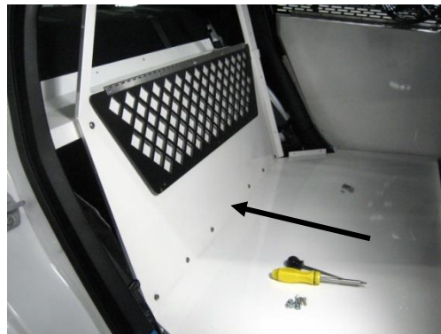
Place rear wall assembly into vehicle. Use 1/4"x 3/4" Phillips pan head machine screws and flat washers to attach rear wall and floor to lower support bracket. Use Awl to help align mount holes through all three parts.
