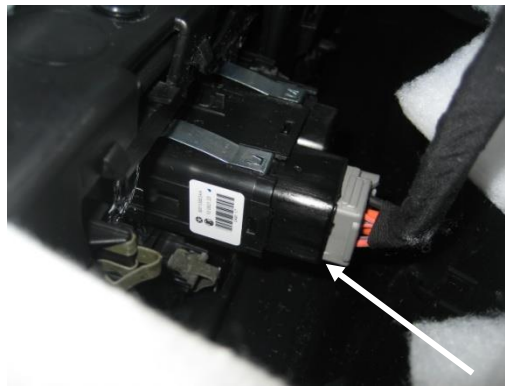
Remove window switch from door panel and reattach it to original plug. Switch must be plugged in for future window operation
