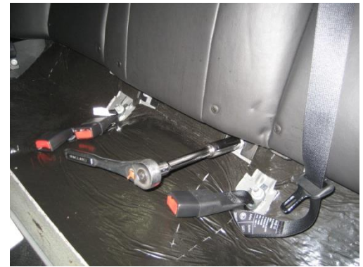
Remove nuts on seat back lower brackets. Save nuts for later use. (18 mm socket)
