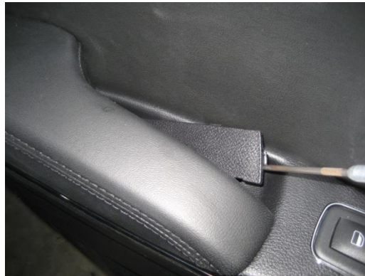
Behind door armrest, remove plastic cover and screw. (Phillips screwdriver) Note: A small 90° scribe (picking tool) helps to take plastic covers off.
