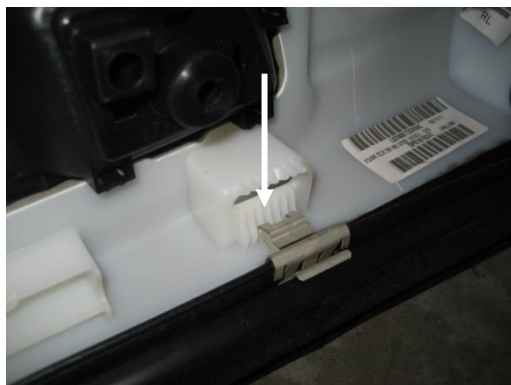
Remove rubber / felt glass wiper edge molding assembly from OEM door panel.
