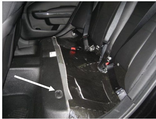
Remove rear seat pad by firmly pulling up on the forward part of pad.
