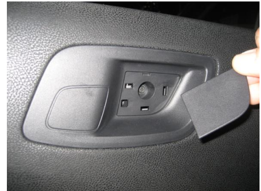
Remove plastic cover and screw at upper area where door release handle would be. (Phillips screwdriver)
